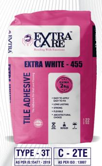
**Extra White-455** is a highly polymer modified cement based thin set mortar used for installation of ceramic tiles, stone, quarry tiles, glass mosaic tiles on most of the substrates to accommodate movements. It is a single component adhesive which can be used for application on both interior and exterior wall / floors.
